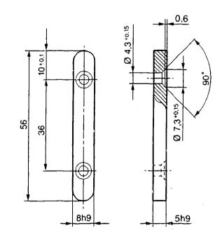
Assembly wrench for threaded ring of multiplate clutch: to be improvised
